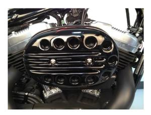
Abb. 1 – Mounted air filter cover "Slotted"
